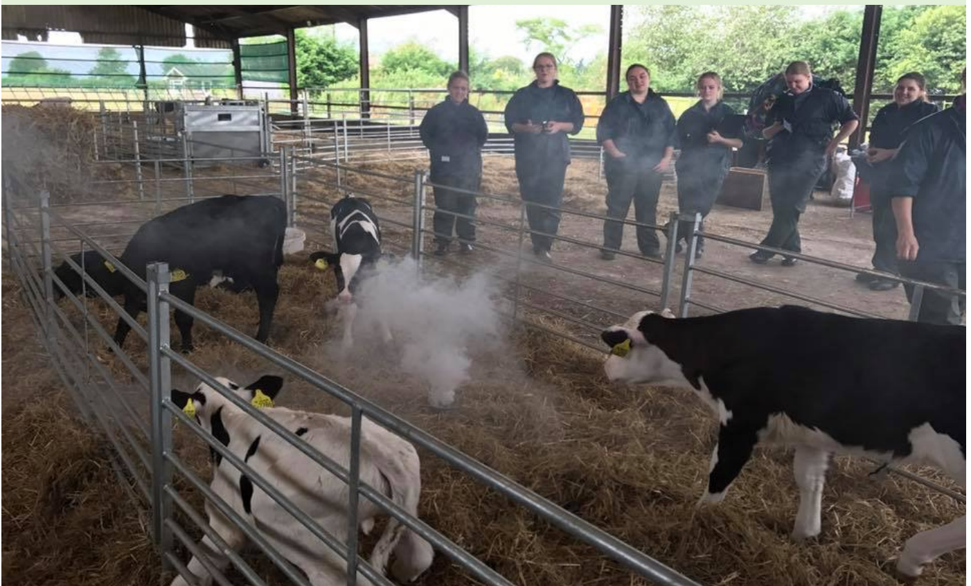
Figure 2: Smoke bomb testing calf shed to look at ventilation. Once the smoke bomb has finished releasing smoke, the smoke should exit the building within one minute. Ideally, fresh air will come in from the sides of the shed and push the stale air (and smoke) to the apex of the roof.
